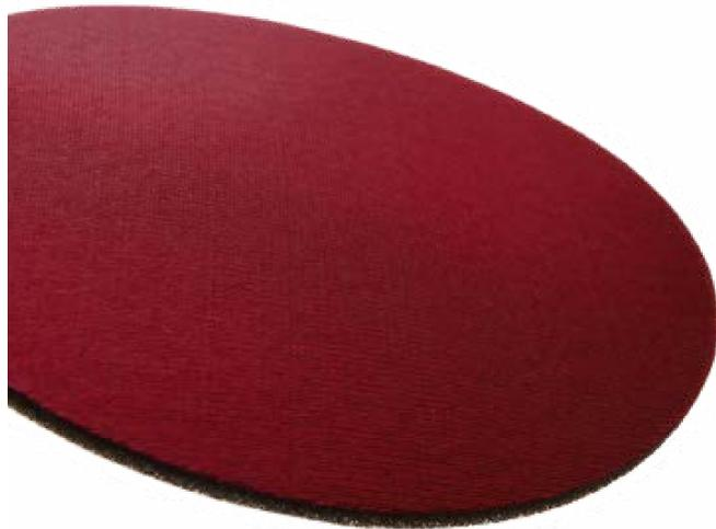
> Sunfoam discs are made up of a soft foam backing laminated with Velsystem, with a layer of structured abrasive. Used with a Velcro backing pad equipped with dust suction, they can sand any non planar surface. The special structured abrasive slows clogging and increases the finish.
